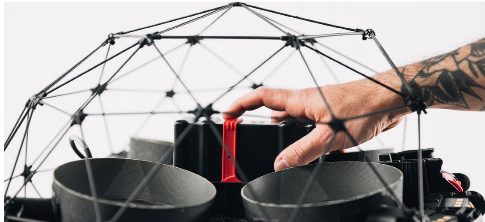
**New insert and lock mechanism to ease battery manipulations**
